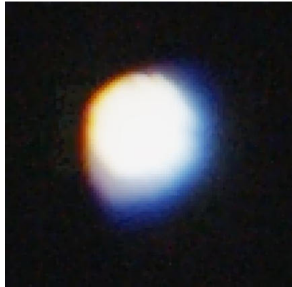
Figure 65. Lateral chromatic aberration of the 100 mm lens. \times 1500 magnified detail of a lateral perforation on the Via Stellae test chart, with slight increases in contrast and color saturation to highlight the separation of the color channels.
