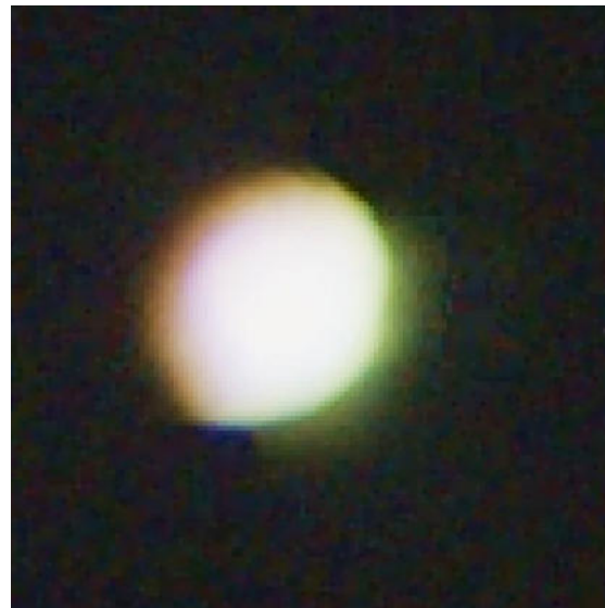
Figure 14. Lateral chromatic aberration of the 35 mm lens. \times 1500 magnified detail of a lateral perforation from the Via Stellae test chart, with a slight increase in contrast and saturation to emphasize channel separation.
