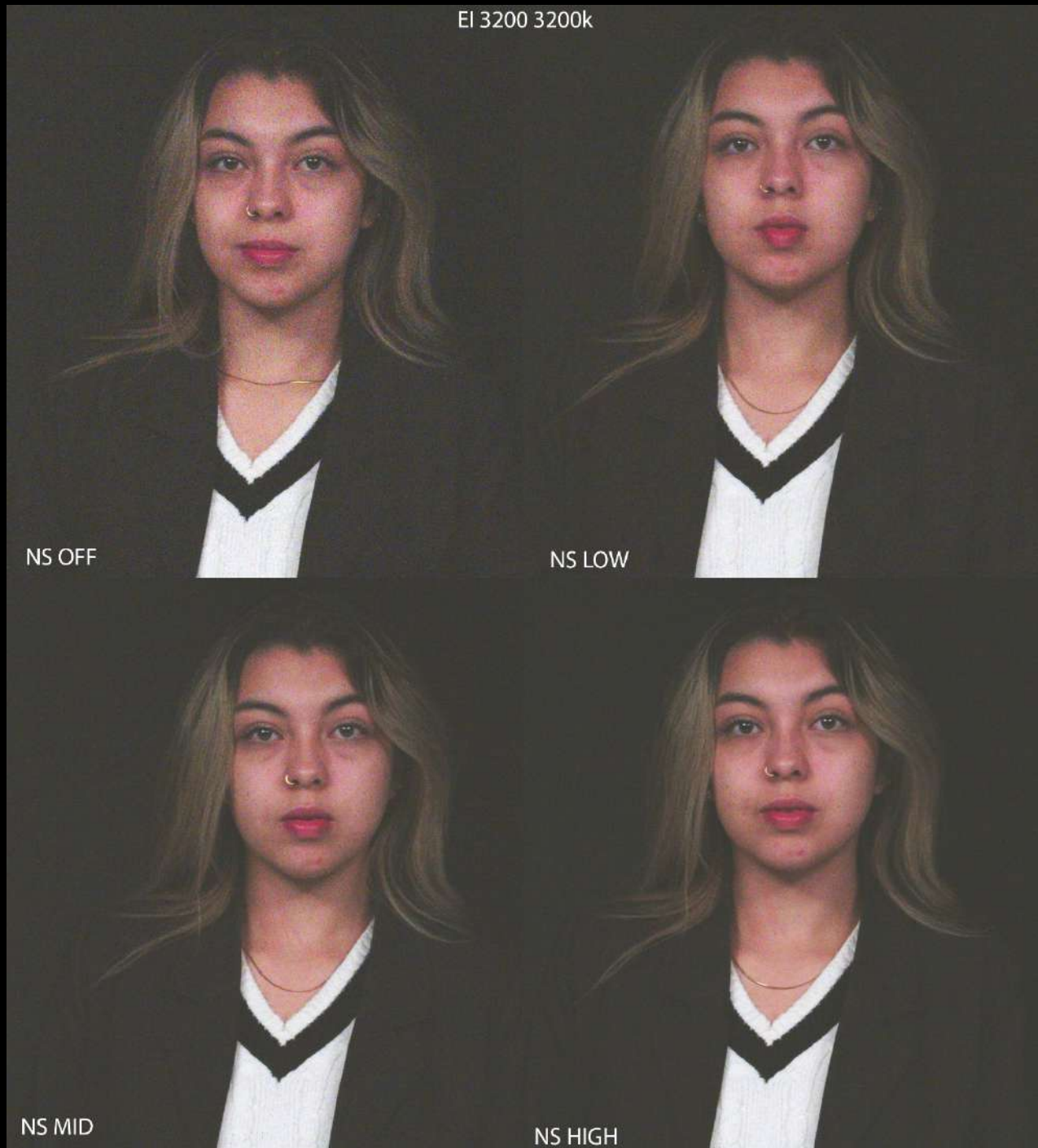
Figure 27. S-Log3 / S-Gamut3.Cine, graded in DaVinci Resolve, with -4 stops of underexposure corrected and converted to Rec.709
