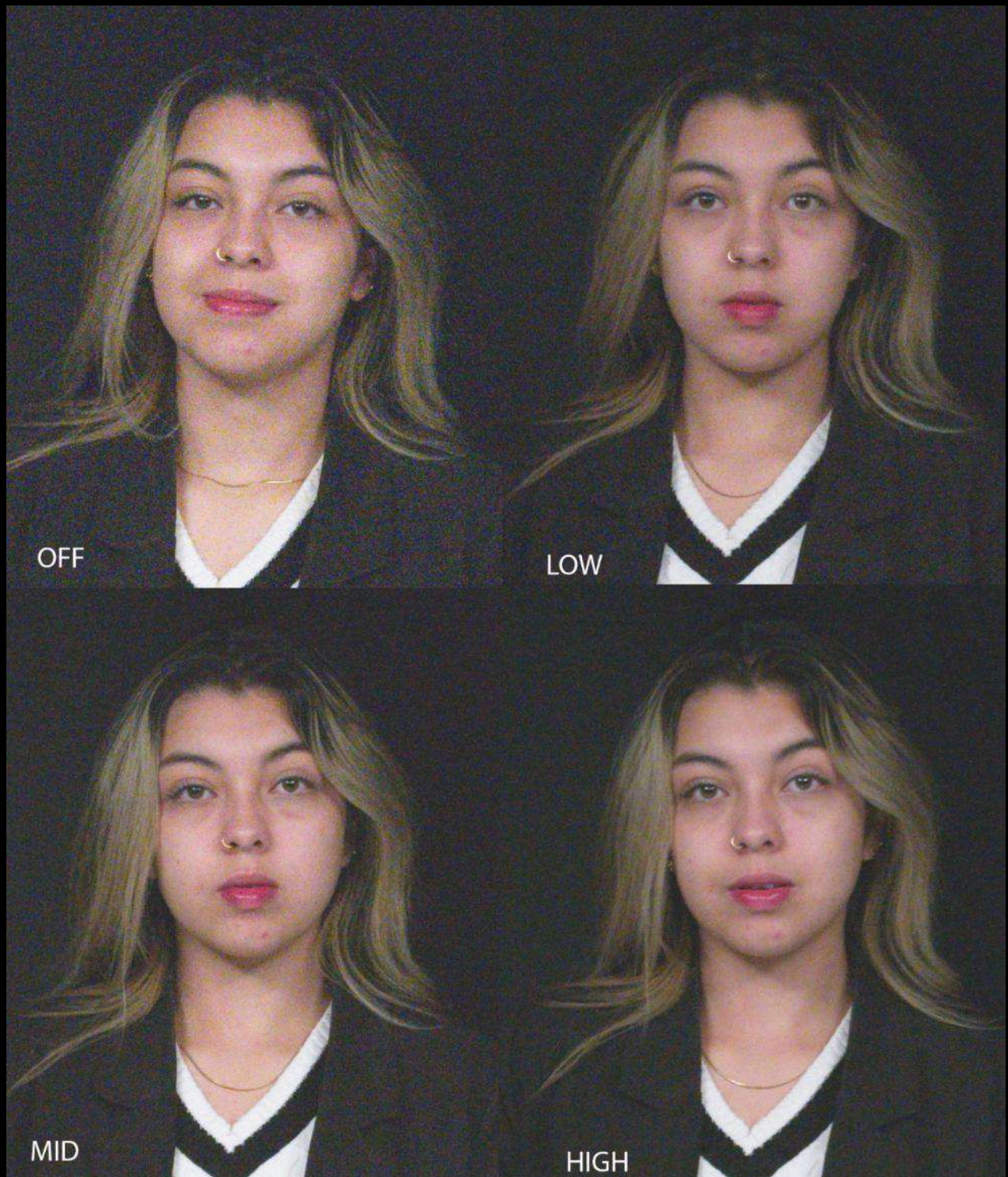
Figure 26. S-Log3 / S-Gamut3.Cine , graded in DaVinci Resolve , with -4 stops of underexposure corrected and converted to Rec. 709
