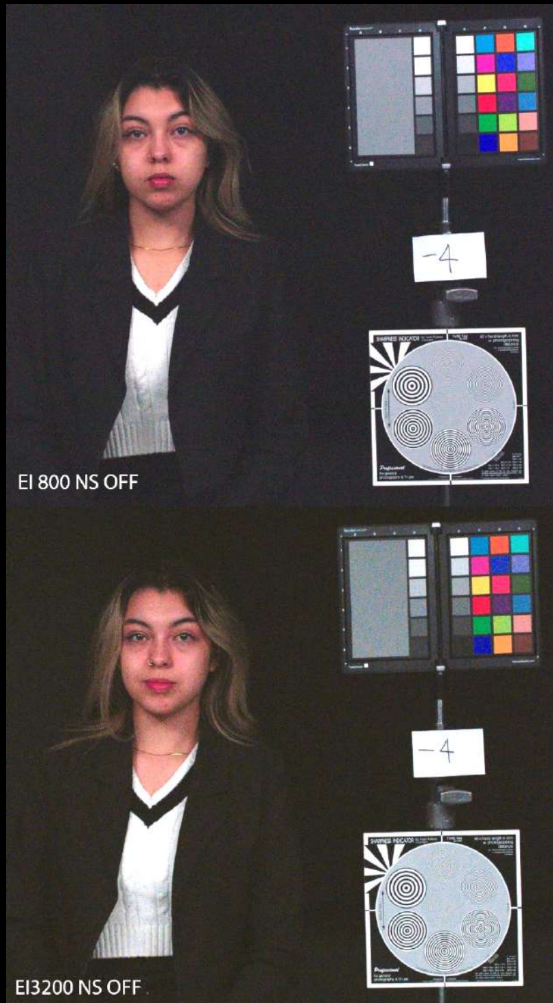
Figure 28. S-Log3 / S-Gamut3.Cine, graded in DaVinci Resolve, with -4 stops of underexposure corrected and converted to Rec.709
