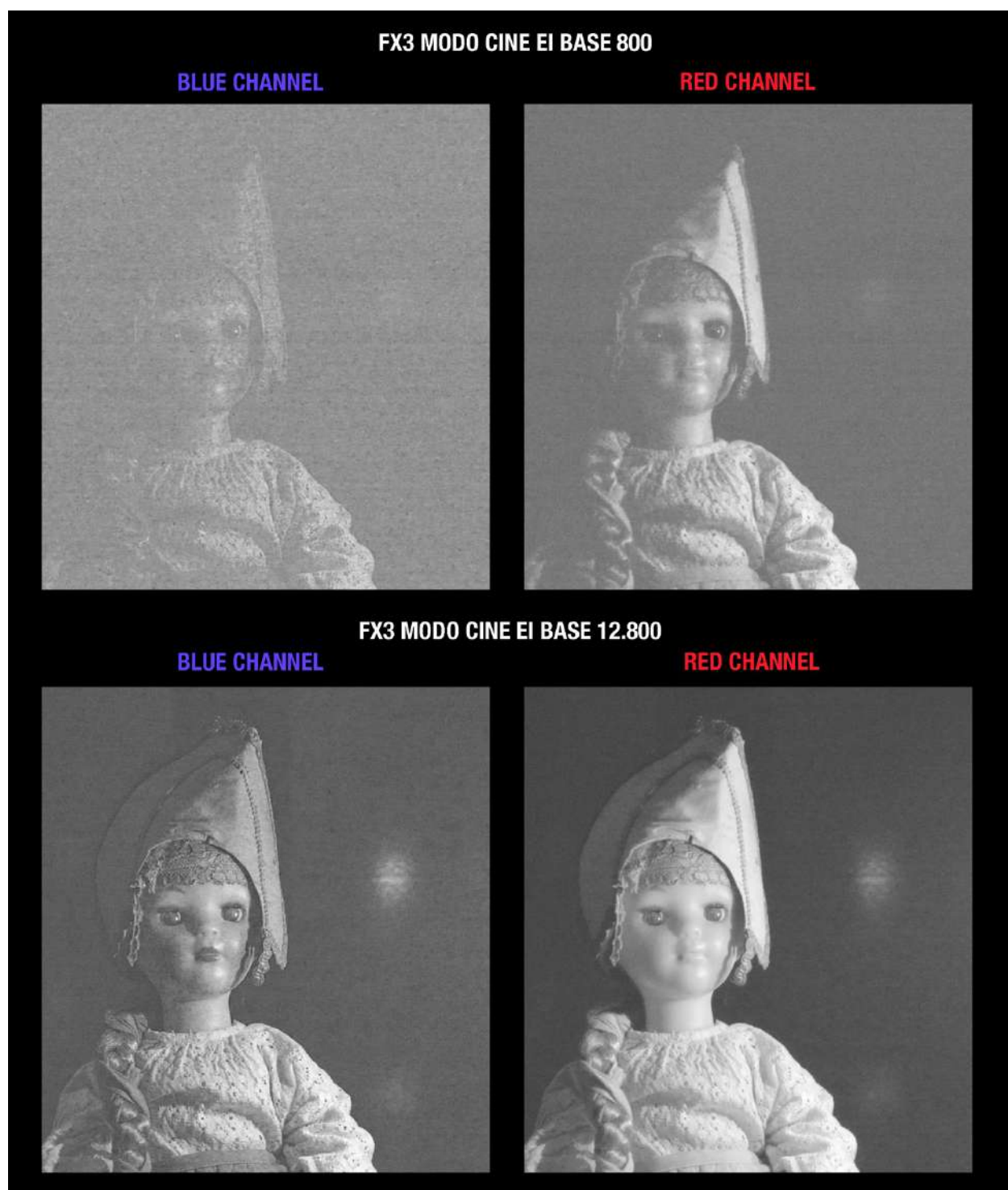
Figure 22. Blue and red channel at two EI Base in CINE EI mode. We have increased the brightness of the channels to better illustrate the differences between them.
