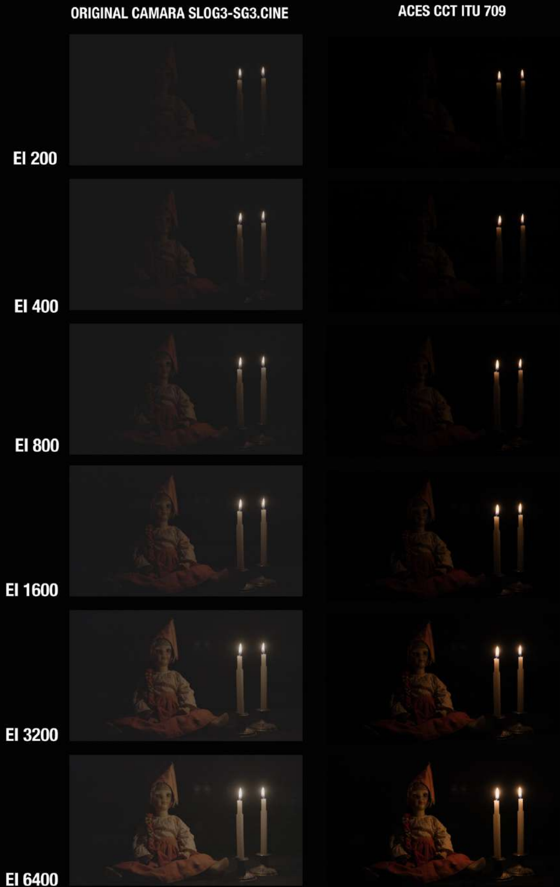
Figure 40. Comparison of flexible Cine EI mode flexible at different ISO values
