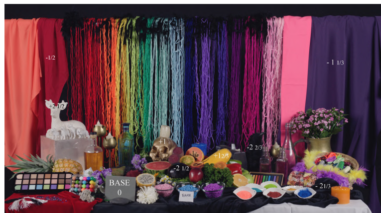
Figure 73. Still life. Some reflectance values in T stop referred to neutral gray 18%
