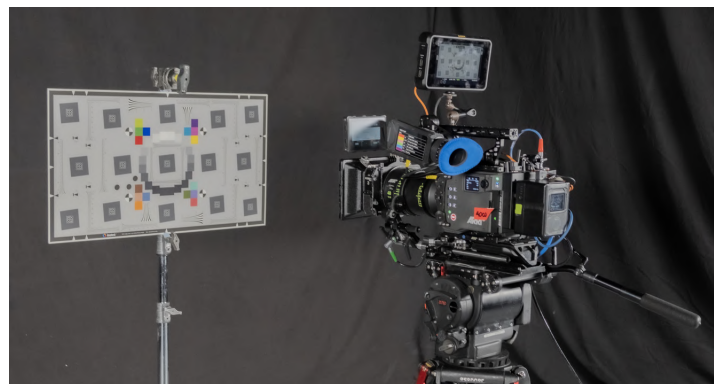
Evaluation of the resolution with the Imatest test chart.
